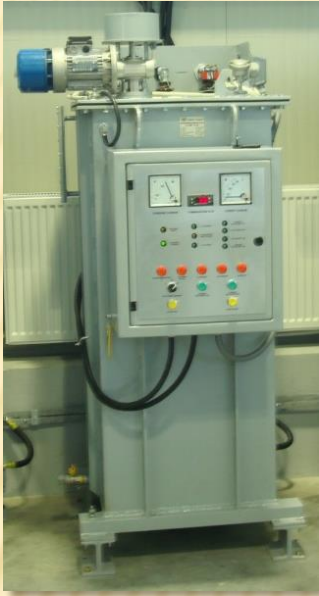
Autotransformer with fine control of the output voltage
